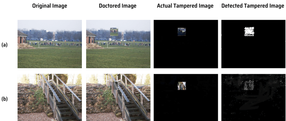
Fig. 3 Results of high quality ghost image inserted into low quality cover image (a) Grass field, (b) Stair
