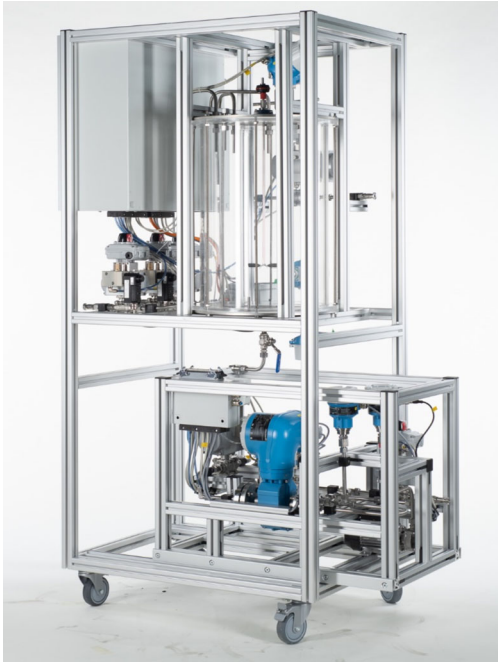
Fig. 4. The reactor-PEA, prepared for FEA exchange
