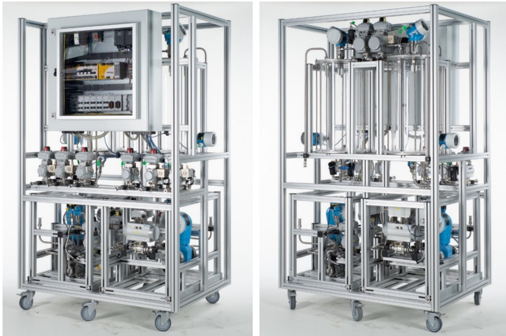
Fig. 3. The double-feed-PEA with view of control cabinet (left) and with view of the vessels (right)
