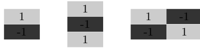
Fig. 1. Rectangle features used by Viola and Jones. The value of a two-rectangle feature is the difference between the sum of the pixels within two rectangular regions. The regions have the same size and shape and are horizontally or vertically adjacent. A three-rectangle feature computes the sum within two outside rectangles subtracted from the sum in a center rectangle. A four-rectangle feature computes the difference between diagonal pairs of rectangles.
