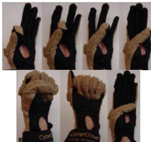
**Figure 6.** Examples of hand positions that may be used for calibration to capture different motions.
