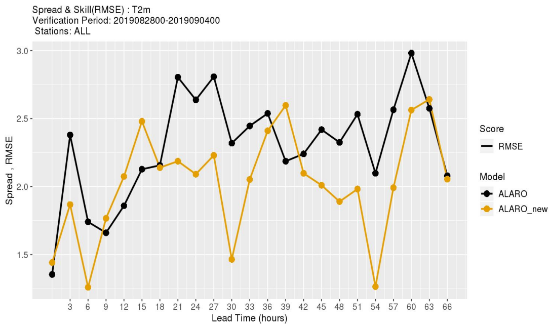
Figure 9: RMSE (top) for 00UTC forecasts of ALARO-PI (left panels with a lead time up to 66-hour) with different initializations: after surface DA (CANARI), yellow line; and without DA, black line.
