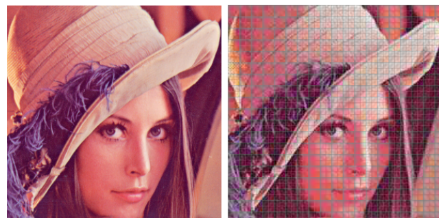
Figure 4: Sample image (on the left) and DST artifacts on block boundaries (on the right).
