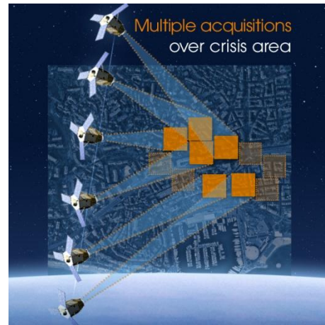
② CMGs allow maximizing numbers of acquisitions over a given area, typically 10 images over an area of 100 x 200 km
