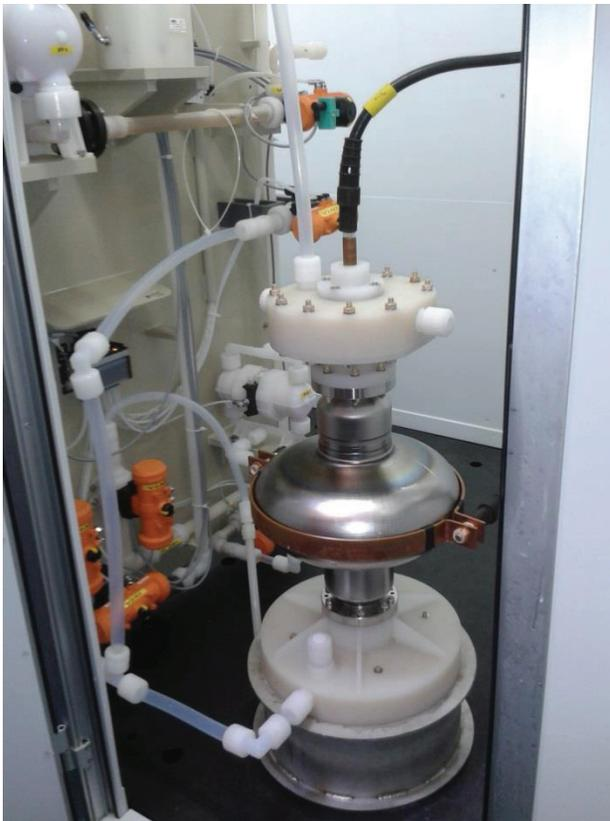
Figure 35: Electropolishing of niobium monocell cavity at CERN.
