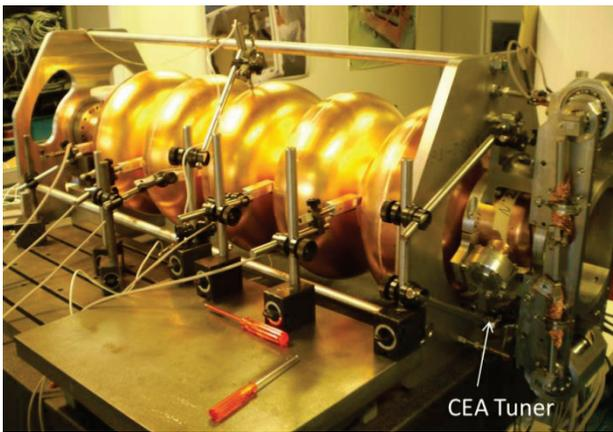
Figure 31: Tests of cavity deformation during tuning with CEA Saclay cold tuner.
