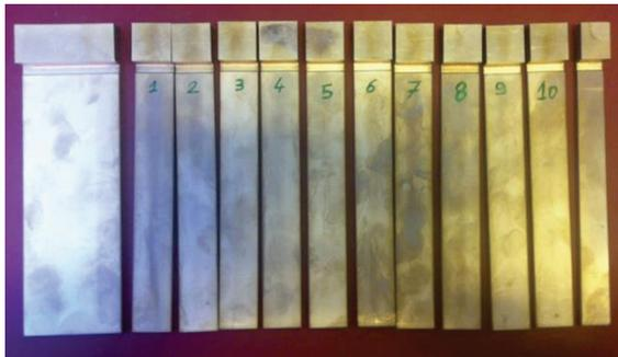
Figure 25: Nb – SS brazed samples for chemical testing.
