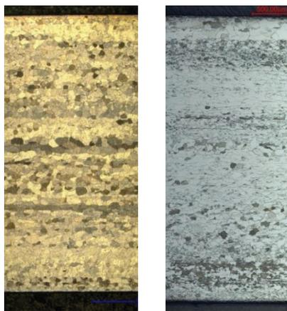
Figure 7: Metallographic observation of Supplier A plate 2 (left) and Supplier B (right).
