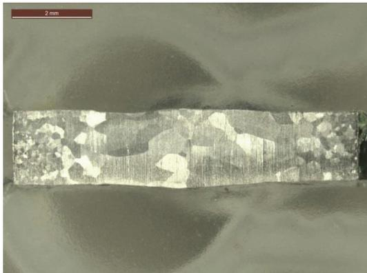
Figure 14: Metallography of a cross section of a linear niobium weld test presenting no defects.
