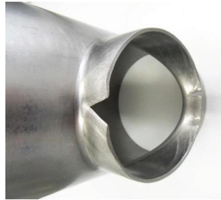
Figure 19: Fractures observed after the necking – out of a port in an end group.
