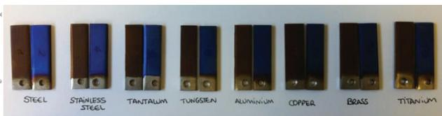
Figure 10: Contaminated and anodised samples for visual inspection.
