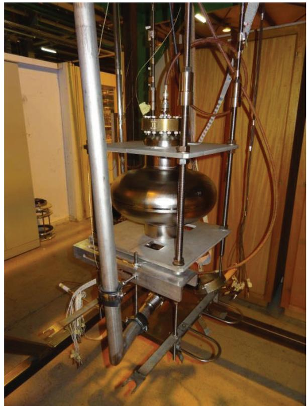
Figure 40: Vertical cryostat for cavity cold test.
