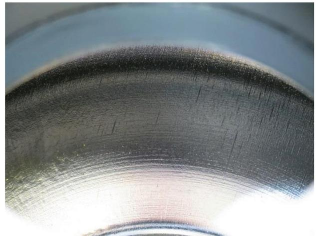
Figure 36: Niobium surface after 220 microns removal by electropolishing.
