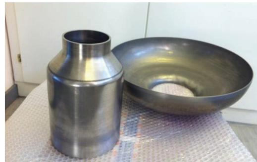
Figure 11: Niobium cavity extremity and half-cell done by spinning.
