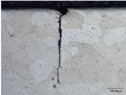
Figure 17: Metallographic observation of a cross section of the defect.
