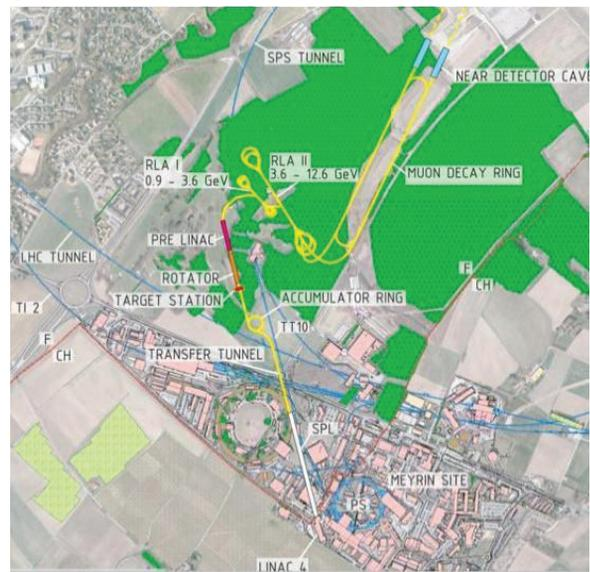
Figure 2: Draft layout of a neutrino factory at CERN.
