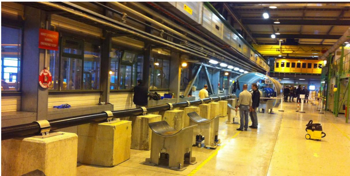
Figure 17: Twenty meter long cryostat of the link (Nexans Cryoflex<sup>®</sup> line) installed in the SM-18.
