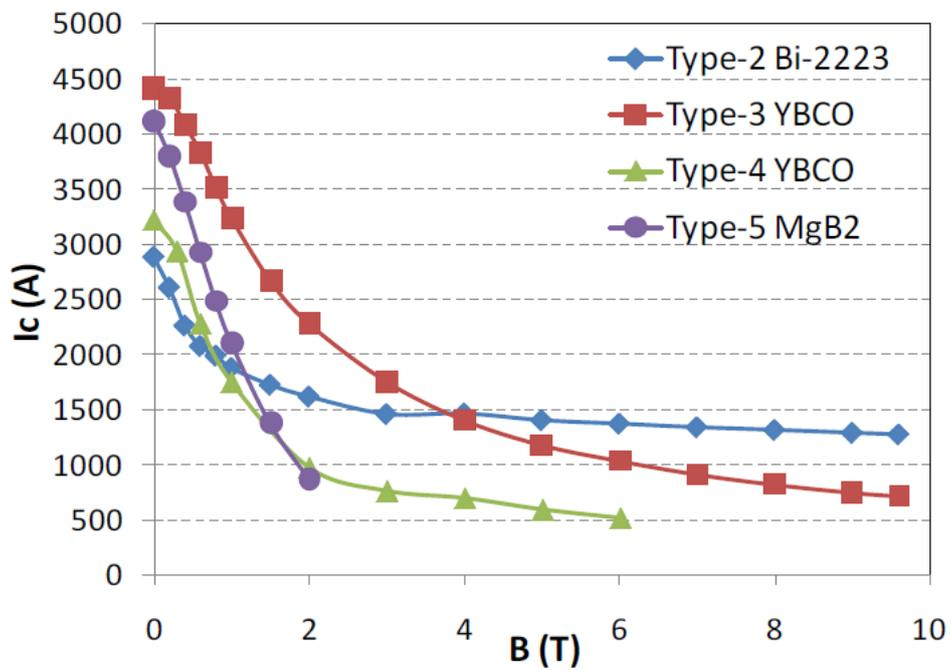
Figure 12:  $I_c$  of one single cable of the twisted pair unit as a function of perpendicular magnetic field at 4.2 K.
