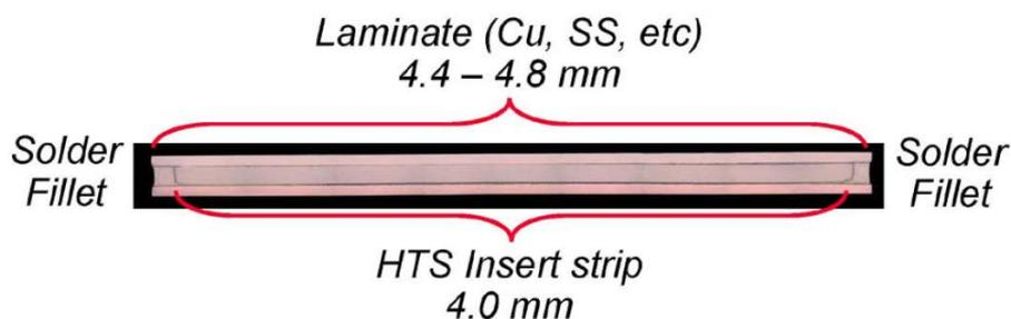
Figure 5: Cross section of YBCO American Superconductor tape.
