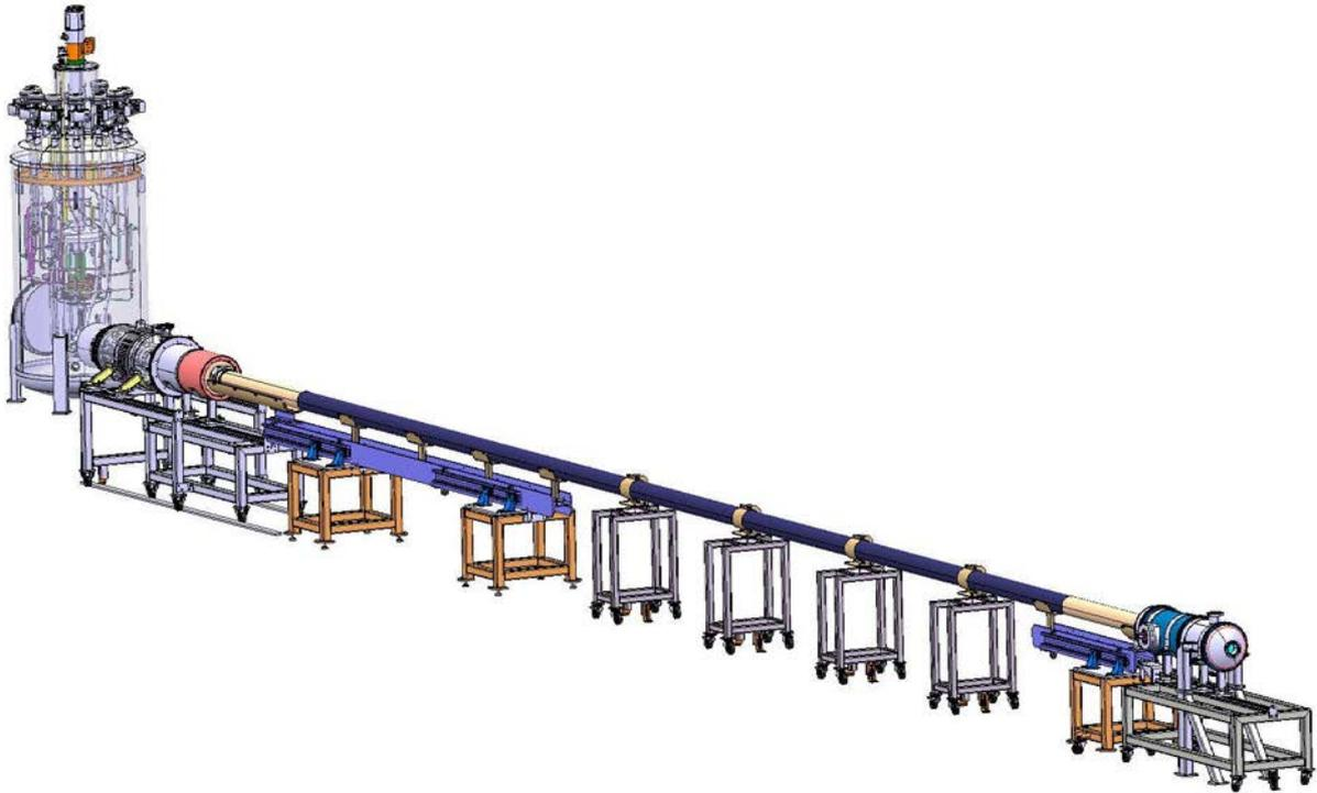
Figure 19: Test station: cryostat with current leads and superconducting link.
