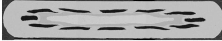
Figure 6: Cross section of Columbus MgB<sub>2</sub> tape.
