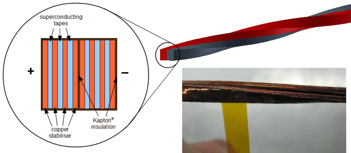
Figure 7: Assembly of twisted-pair cable unit.
