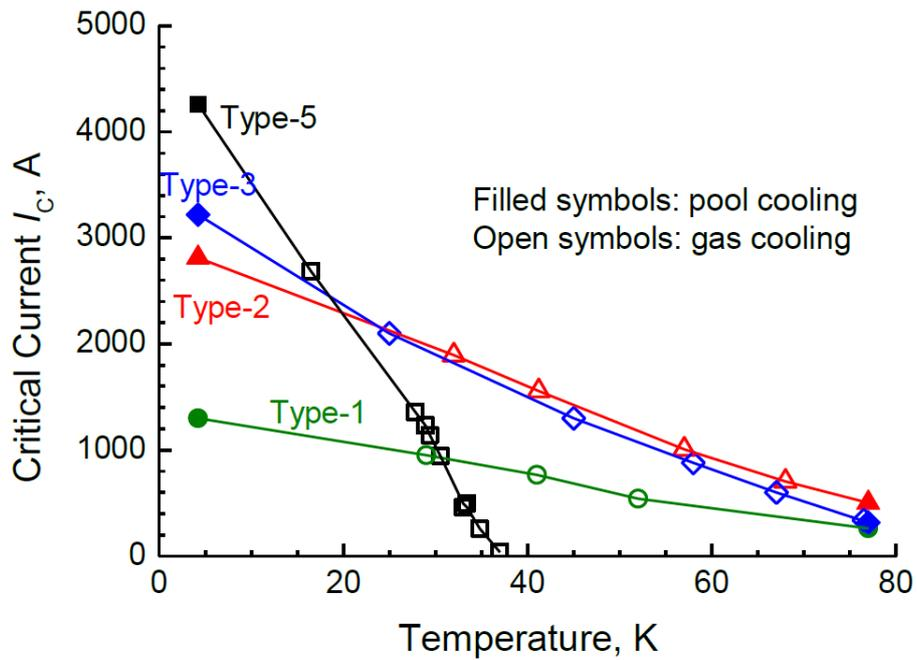
Figure 14: Critical current as a function of temperature measured on one cable of the twisted-pair unit [8]. The correspondence between the Type-n cable and the type of conductor is reported in Table 1.
