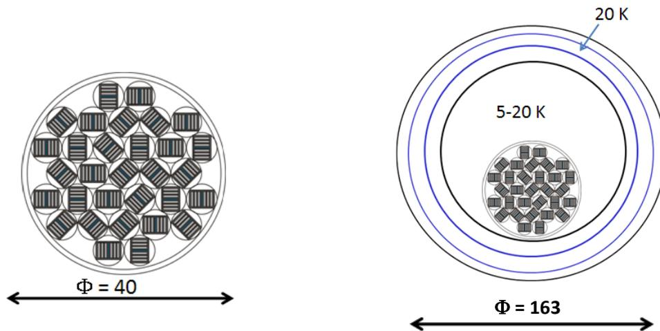
Figure 9: multi-cables assembly of 24 twisted-pair cables (left) and cryostat with the cable (right).
