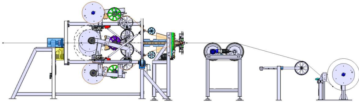
Figure 16: Rotating machine for the twisting of the insulated stacks of the conductor – assembly of twisted-pair cables.
