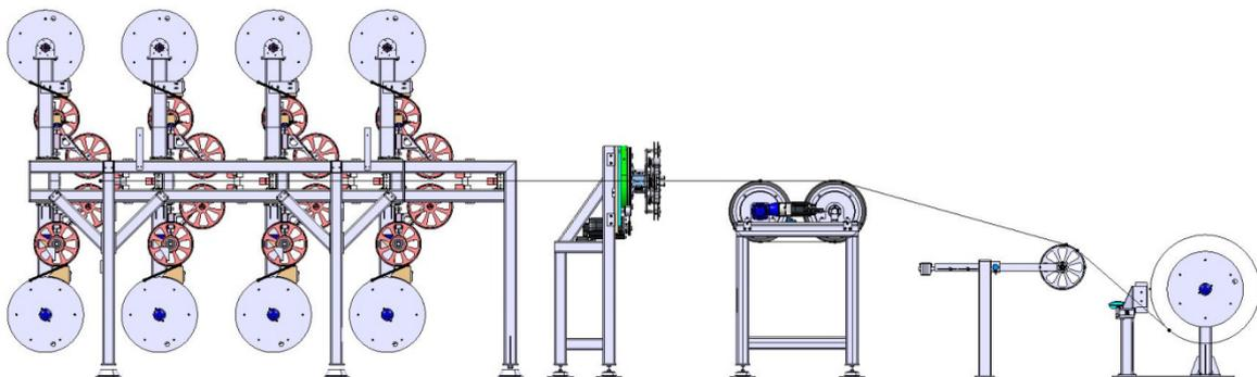
Figure 15: Static machine for the assembly of insulated stacks of tape conductors.
