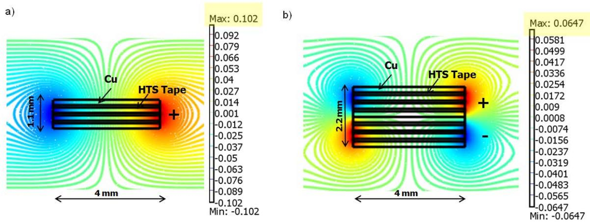
Figure 8: Perpendicular self-field component in one 600 A cable (left) and in a twisted pair of 600 A cables (right). Colour scale: Max: red, Min: light blue.
