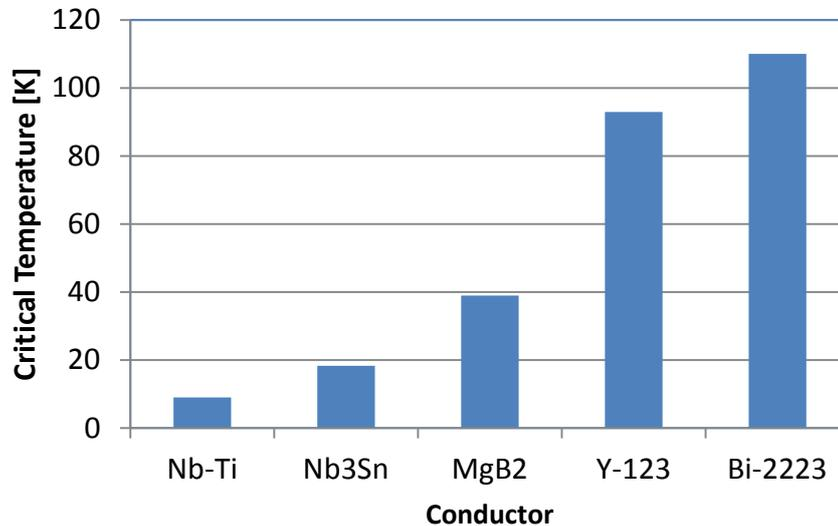
Figure 1: Critical temperatures of superconductors.
