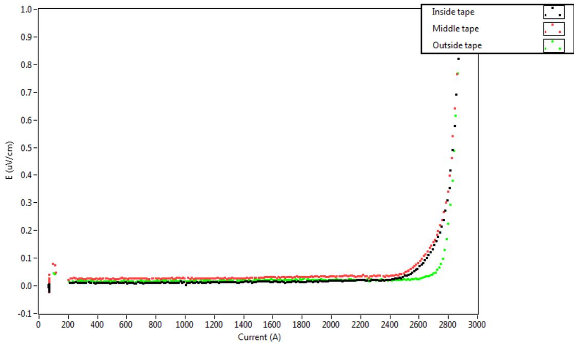
Figure 11: E-I curve measured at 4.2 K and in self-field on each of the 3 tapes in a single cable of a Bi-2223 (Sumitomo) twisted pair unit.
