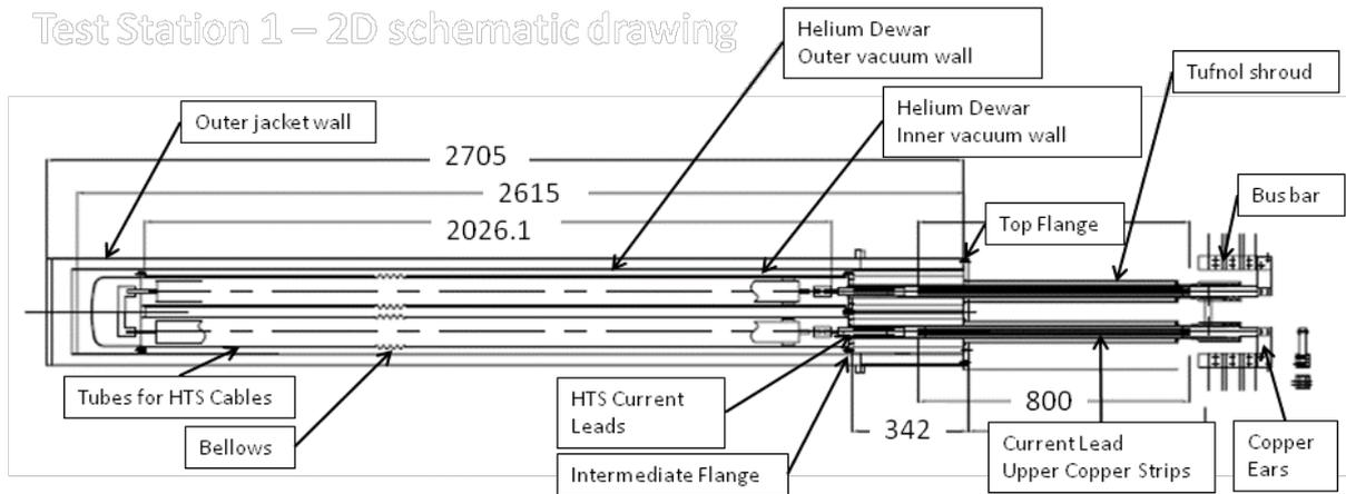
Figure 13: Cryostat built for the measurement of the twisted pair cables in He gas in a variable temperature range.
