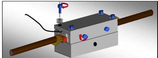
Figure 1: Design of an oven for resistive soldering
