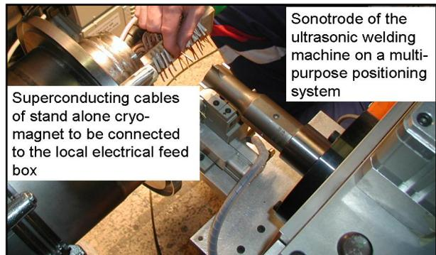
Figure 2: Ultrasonic welding in the special IC
