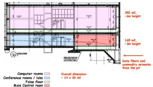
Figure 4: CMS DAQ building at experimental site
