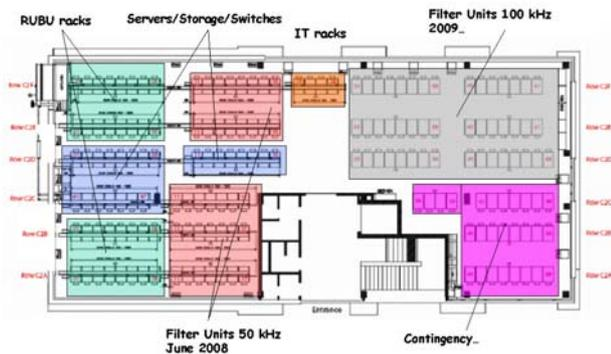
Figure 6: Rack layout in CMS computer room
