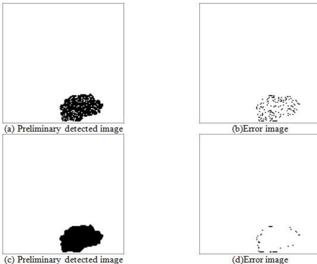
FIGURE 8. (a) detected image without refinement mechanism under the second scenario, (b) error image without refinement mechanism under the second scenario, (c) detected image with refinement mechanism under the second scenario, (d) error image with refinement mechanism under the second scenario
