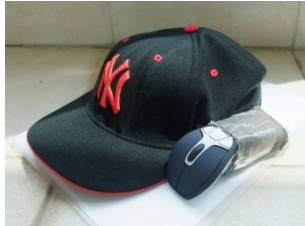
Fig. 3. Wireless gyrometer sensor attached to a cap
