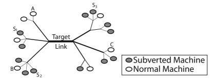
Fig. 1. Example Network Where Coremelt Would Succeed (Note: Line thickness indicates available bandwidth)
