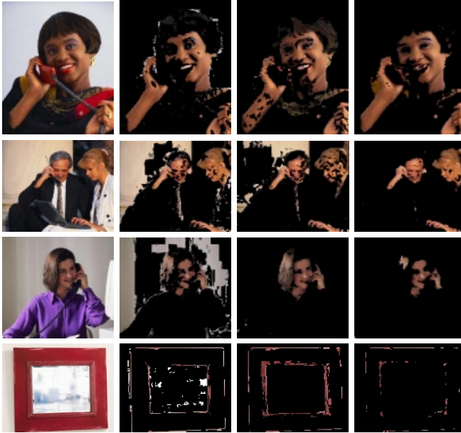
Fig. 5. Examples of results of skin color detection using (from the left to the right) the methods proposed in [11], in [28] and in this paper with the variables (L, a, b) .
